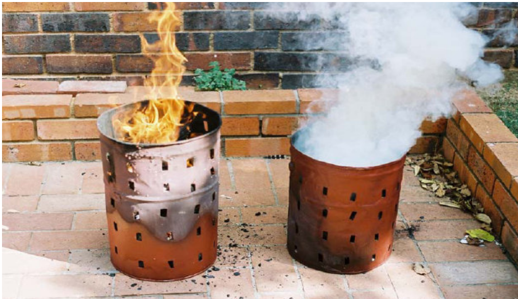
Figure 9: Smoke emissions using traditional D-grade coal from the Basa njengo Magogo fire (left) and a conventional fire (right) (Wagner et al. , 2005)
